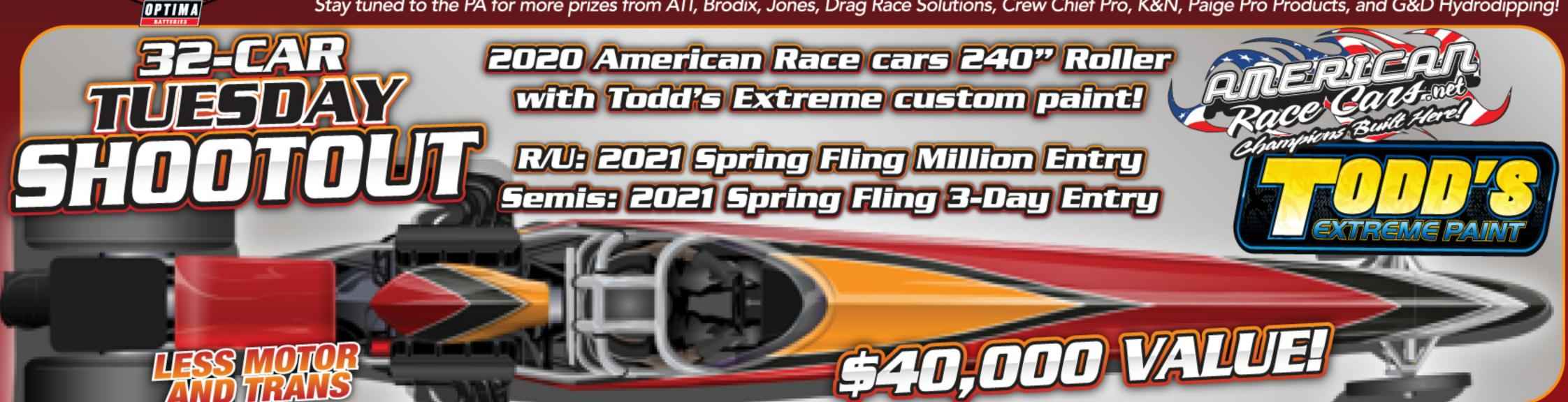
240" Powder-Coated American Race Cars Chassis • Custom Paint Job by Todd's Extreme Paint • Complete Moser Rear-End with Dual Brakes & 40-Spline Axles & Aluminum Center Section • Complete Heavy Duty Drive Shaft with Yoke and U-Joints • Saldana Radiator (on the blow shield) • Complete Dual Brake Package Plumbed with Master Cylinders • Hand Brake and Flex Lines in the rear RBZ Custom Billet Wheel
